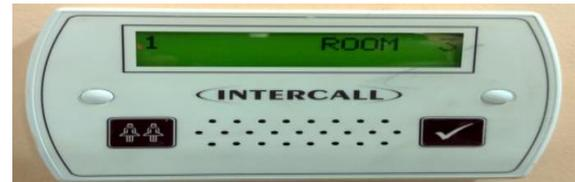
Figure (3) call from room No 3 arise in the display unit
