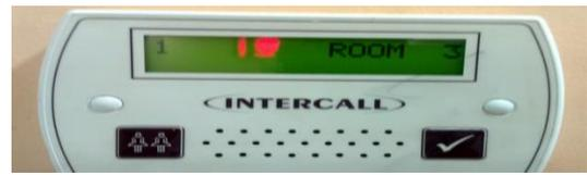
Figure (12) alarm will arise as speed red flash and different alarm voice
