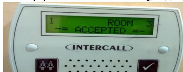
Figure (5) nurse get the number and press “accepted” after that, the alarm voice will stop automatically and the light of the over the door and the slave /master call point will change from red to the green flash light, and that as a response for the patient as shown in Figure (6).
