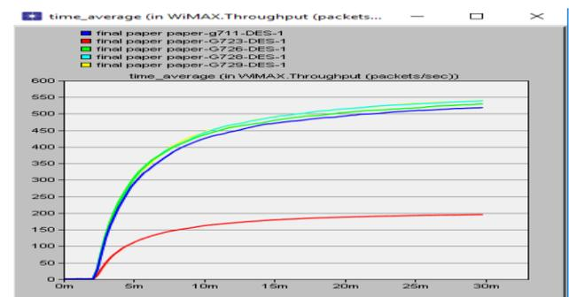
Figure 5-3: WiMAX Throughput (packet/sec)
