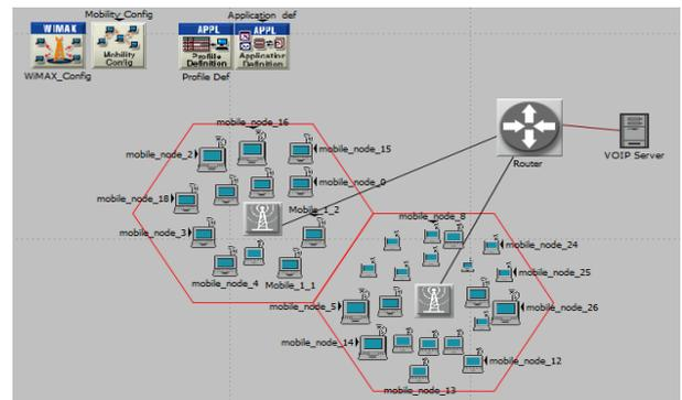
Figure.3 Network Structure topology using OPNET for simulation
