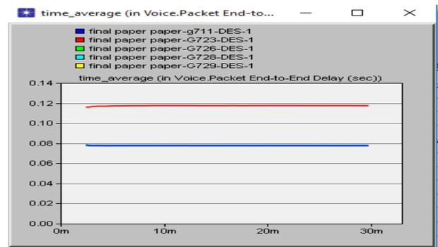
Figure. [4-4] Packet End-to-End Delay (sec)
