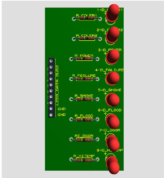
Figure 7. 3D Layout of Display Unit
