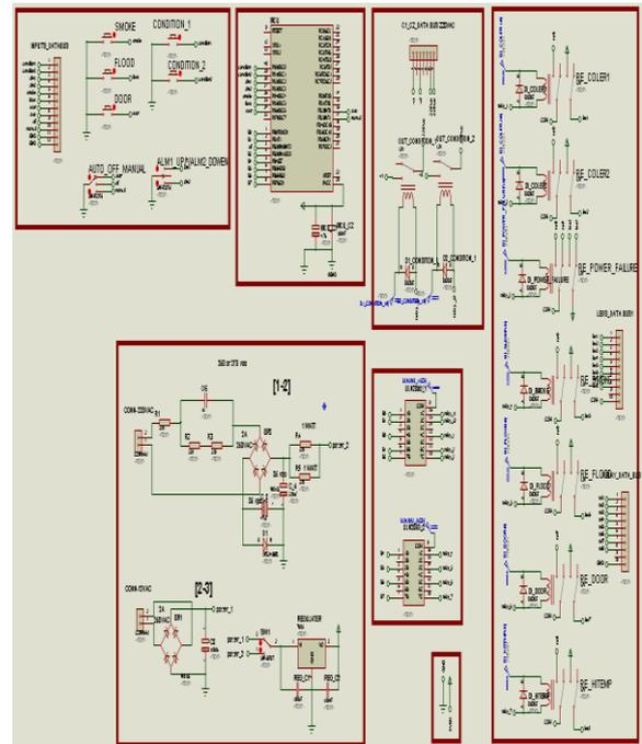
Figure 5. Alarm and Switching Controller for Air Condition Units Schematic
