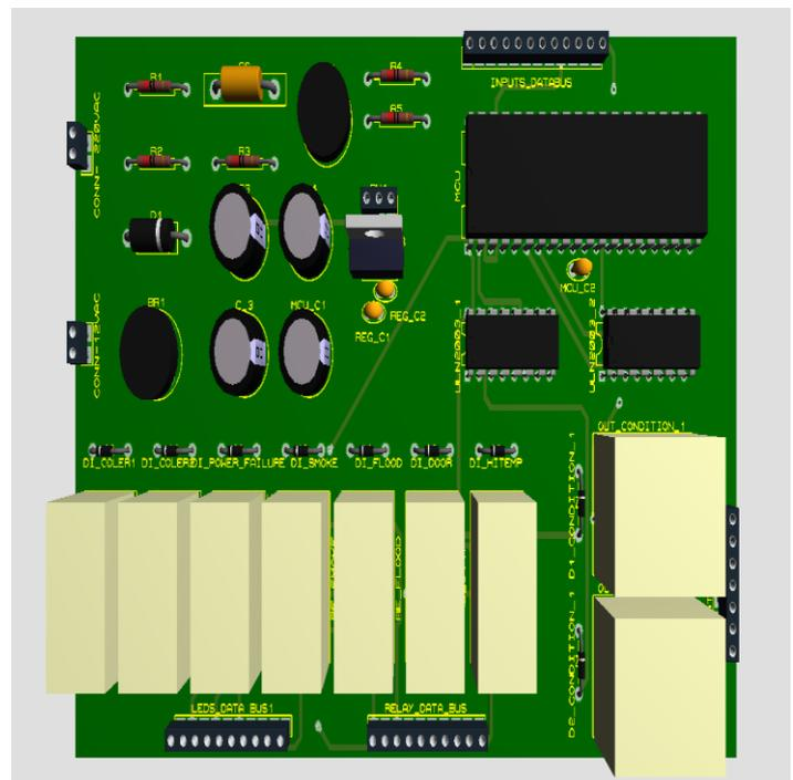
Figure 6. 3D Layout of Main Control
