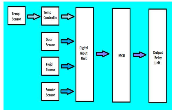
Figure 1. Flow chart of the Alarm and Switching Controller
