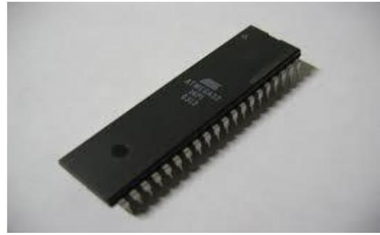
Figure 3. Microcontroller (ATMEGA32)
