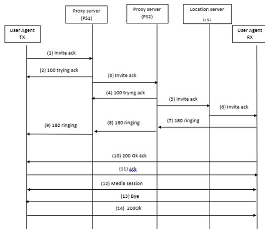
Figure (1) the SIP signalling
