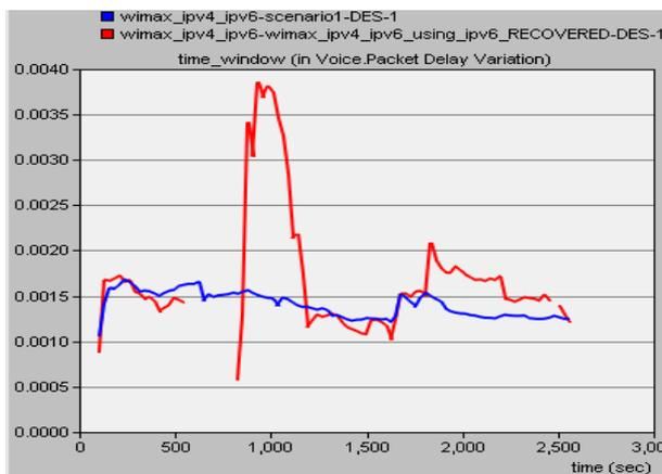
Figure 6: IPv4 vs. IPv6 (blue curve is IPv4, red curve is IPv6) packet delay variation, the packet delay variation of Pv4=0.00140361238041 (1.4036ms) and for IPv6= 0.00168223661794 (1.683ms)
