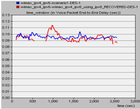
Figure 4: IPv4 vs. IPv6 (blue curve is IPv4, the red curve is IPv6) packet end-to-end delay, the delay mean for IPv4=0.0953489929312 (95.3ms) and IPv6=0.0943925674727(94.3ms)
