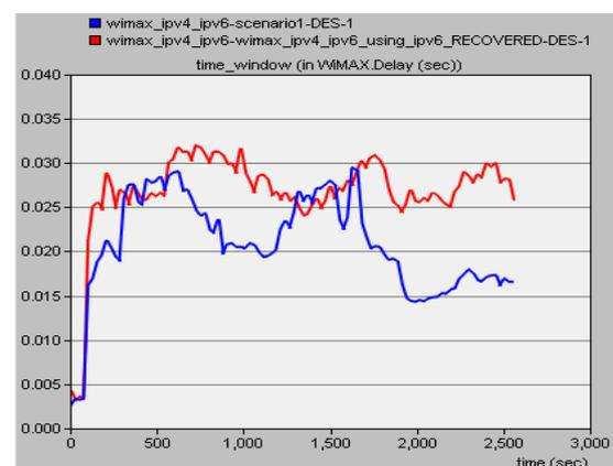
Figure 3: IPv4 vs. IPv4 (blue curve is IPv4, the red curve is IPv6) delay, the delay time mean of IPv4 =0.0207106209876 sec (20ms) and for IPv6 =0.0266530812287 (26.6ms)
