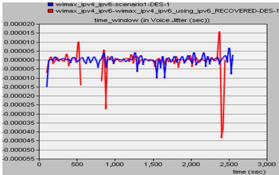
Figure 5: IPv4 vs. IPv6 (blue curve is IPv4, the red curve is IPv6) jitter, the jitter mean for IPv4=-3.64249390875E-007 and for IPv6=-1.39077861152E-006
