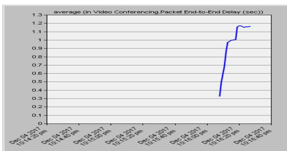
Figure 9: video Packet Delay
