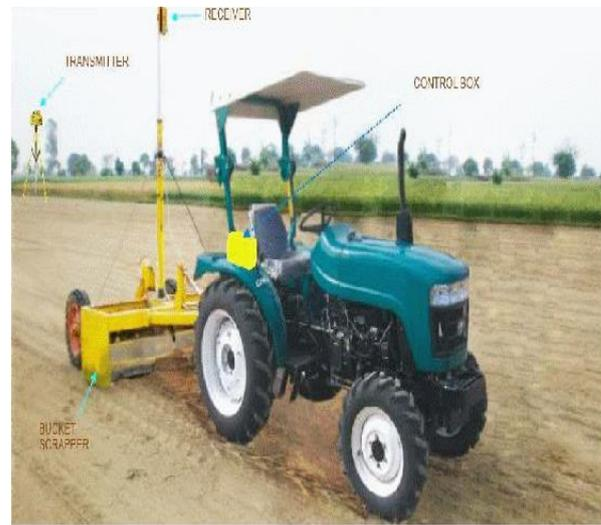
Figure 1: Land Leveling Device Using Laser Technology
