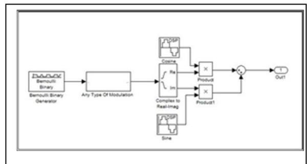
Figure 1 Primary User Block in Simulink
