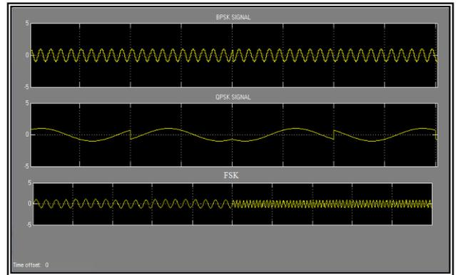
Figure 10 Primary user signal using BPSK, QPSK and FSK
