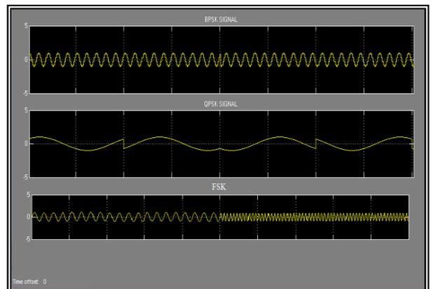
Figure 11 Secondary user signal using BPSK, QPSK and FSK
