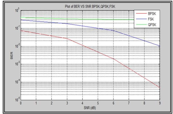
Figure 9 Comparisons between BPSK and QPSK and FSK
