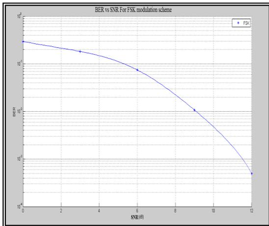
Figure 8 ER vs. SNR use FSK modulation
