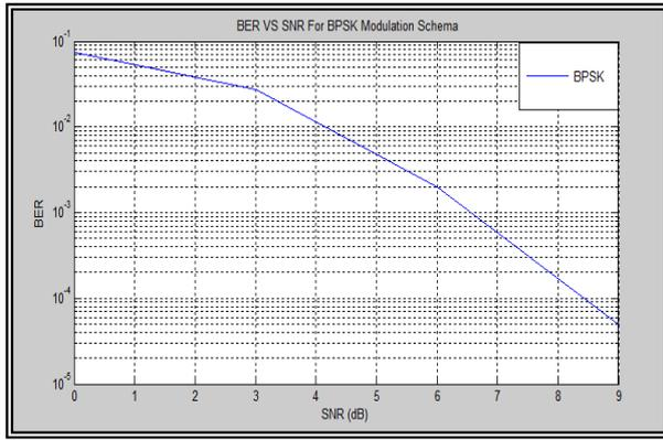
Figure 6 BER vs. SNR use BPSK modulation
