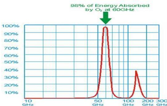
Figure2: Oxygen Absorption at 60GHz
