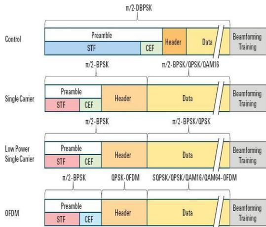
Figure 1: Structure of three modulation types
